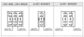
1,2,3,4 are one set;1,2 are normal closed(NC);3,4 are normal opened(NO). The standard LED terminals have no difference of anode and cathode. The lamp and switch are relatively independent and can use switch or peripheral circuit to control the lamp state.
